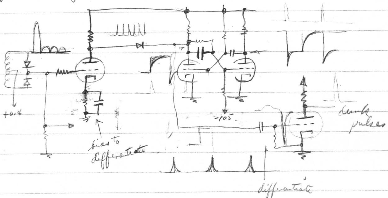
may need phase inverter to trigger with neg pulses
