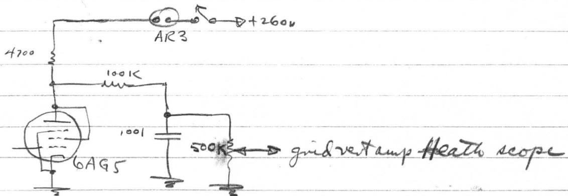
2/2/65 Since  $\Gamma$  correction based on envelope feedback is limited by the demodulator time constant, a diode approach may be better.
