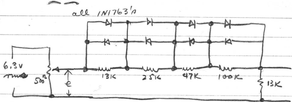
output looks good for  $e = 1.75V_{rms}$  or  $2.5V_{peak}$   $5V_{p-p}$
