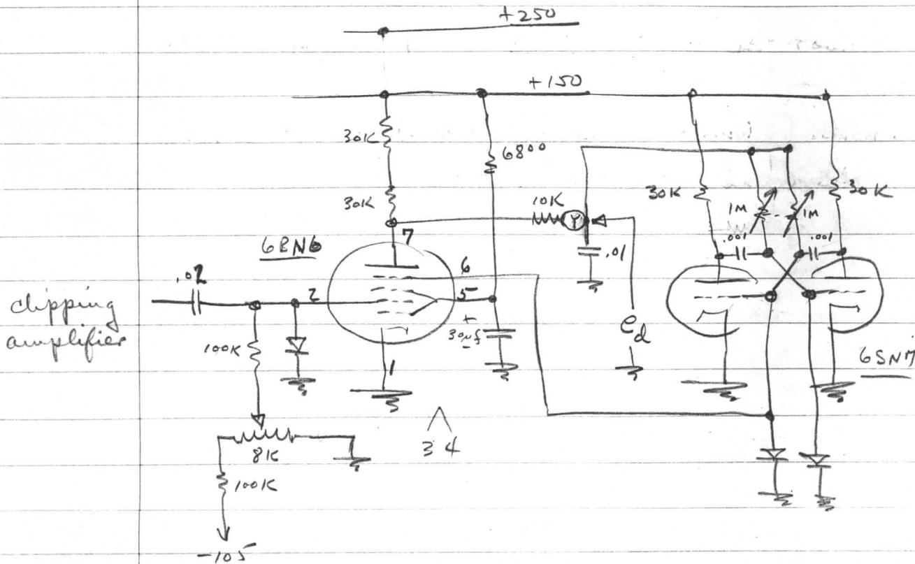
$$\frac{e_d}{q} = \frac{90v - 53v}{180^\circ} = \frac{36v}{\pi} = 11.5 \text{ v/radian}$$
