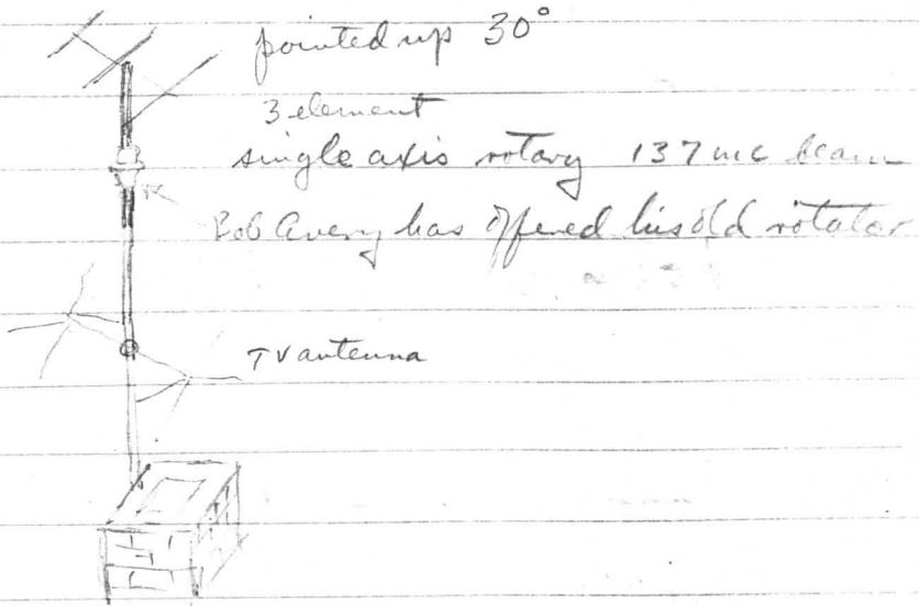
Installation to give signals for RF experiments. To set up the beam, I need VSWR bridge and signal source.
